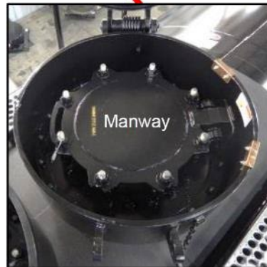
Manway with hinged and bolted manway cover
