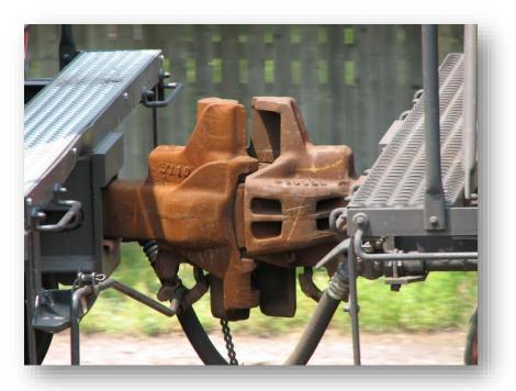
Double Shelf Coupler All Tank Cars Hazmat/Non-Hazmat
