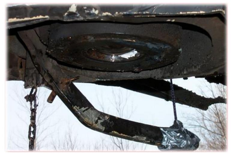
BOV w/ Skid Protection – Ball Valve Intact
